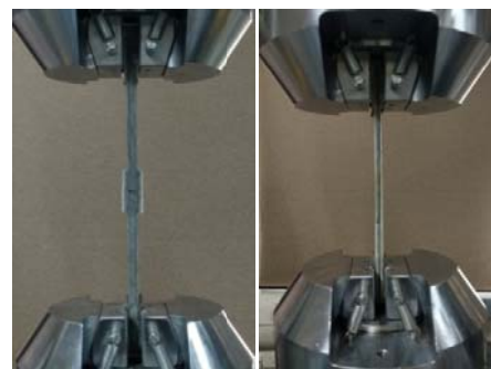
Fig. 2 Double-strap joint and single lap joint specimen placed in UTM.
