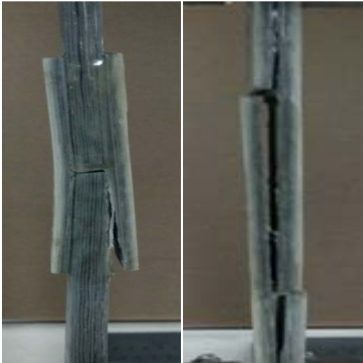
Fig. 7: The thin-layer cohesive (TLC) or light-fiber-tear (LFT) failure observed in test
